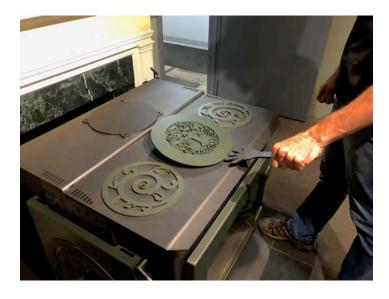
3. Lift the top lid and remove the radiator. The radiator shrouds the catalytic combustor.
