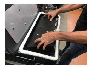
4. Lift the catalytic combustor up and out of the stove.
