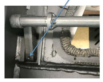
8. Using the t-handle Allen wrench turn the set screw counter-clockwise until the set-screw is removed. With the set screw removed, the outer handle and the inner bypass rod can be separated.
