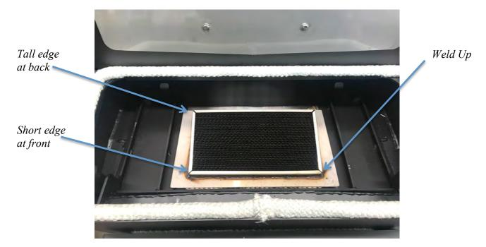
13. Replace the radiator. The standoffs will go towards the back of the stove, and the radiator shield attachment will be at the front of the stove.
