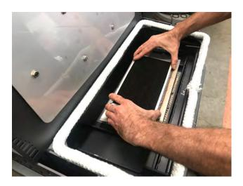
5. Position the bypass handle so that it is parallel to the floor.
