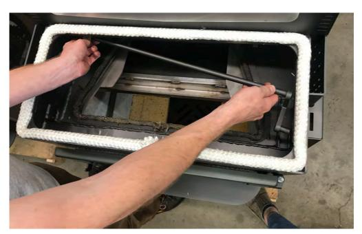
11. Place the sled back into the stove making sure the sled hooks attach to the bypass rod. The hooks will be on the outside of the two round washers welded onto the bypass rod.
