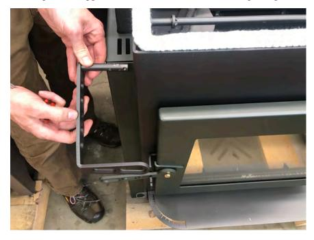
10. To remove the inner rod assembly angle one side of the rod towards the rear of the stove, then lift the front edge of the rod assembly out.
